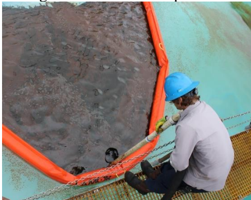
Figure 7 – J-trap Vacuum Skimmer
