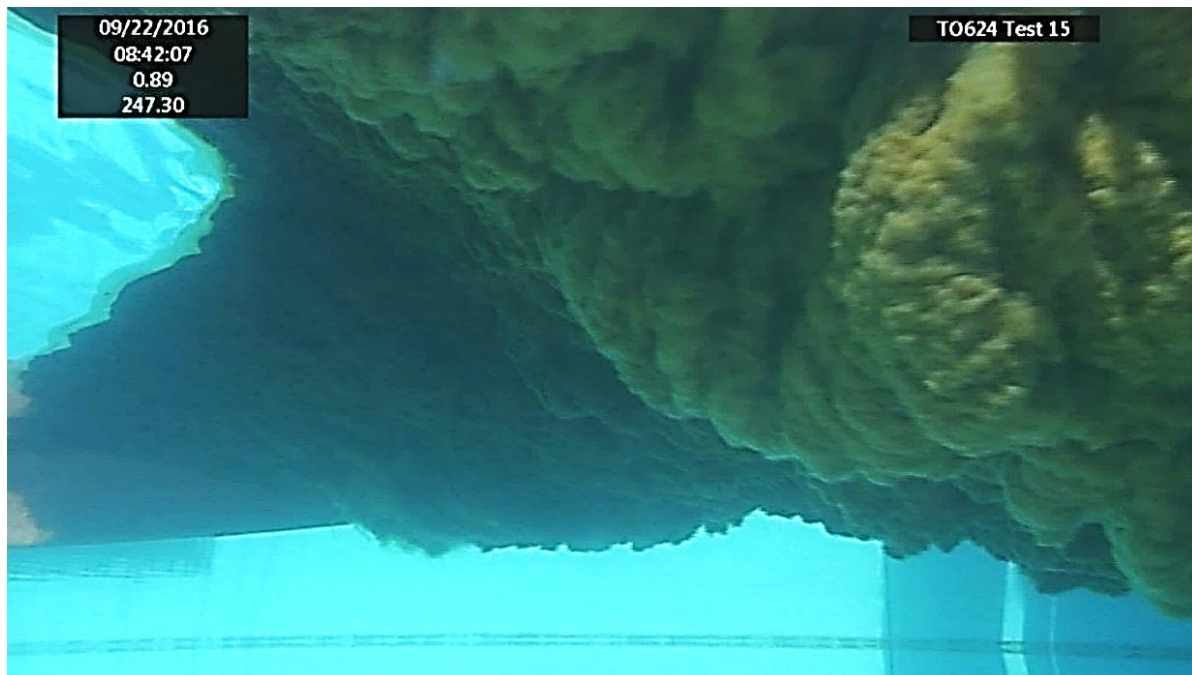
Figure 14 – Underwater View of Oil Dispersing and Flowing Under Boom – DOR 1:50
