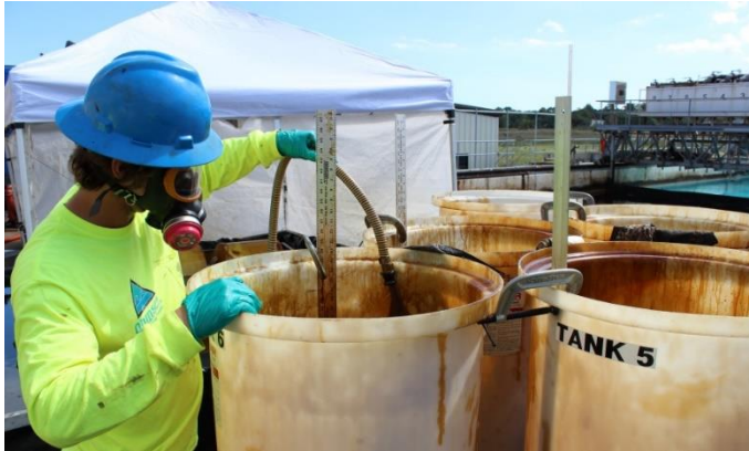
Figure 11 – Timing a Drum Skimmer Test
