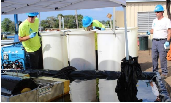
Figure 11 – Timing a Drum Skimmer Test
