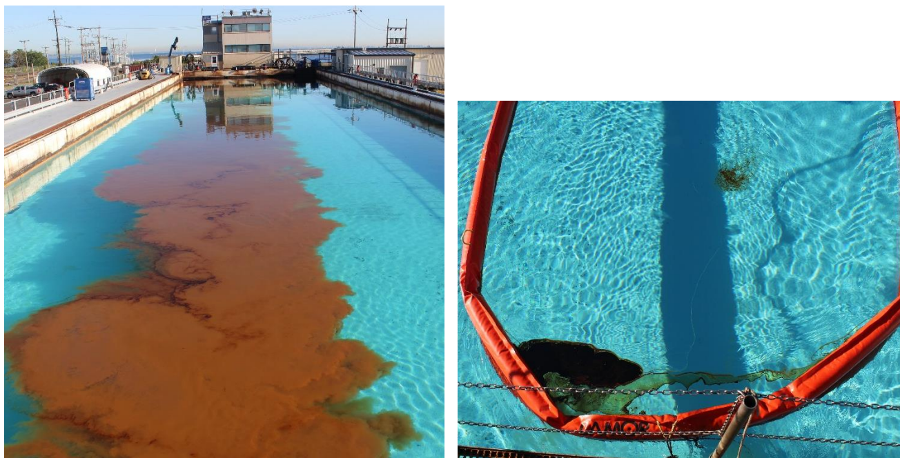
Figure 15 – Oil Dispersed Behind Boom (left) and Remaining after DOR 1:50 test (right)
