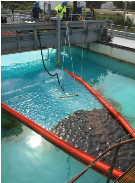
Figure 6 – Containment Boom and Oil Distribution Bar
