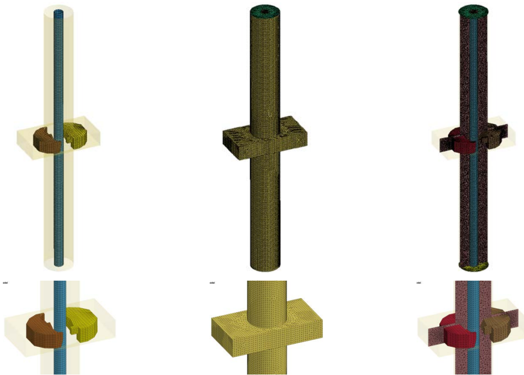
Figure 2-42. Tier 4 FEA and CFD Simulation Discretized Domains
