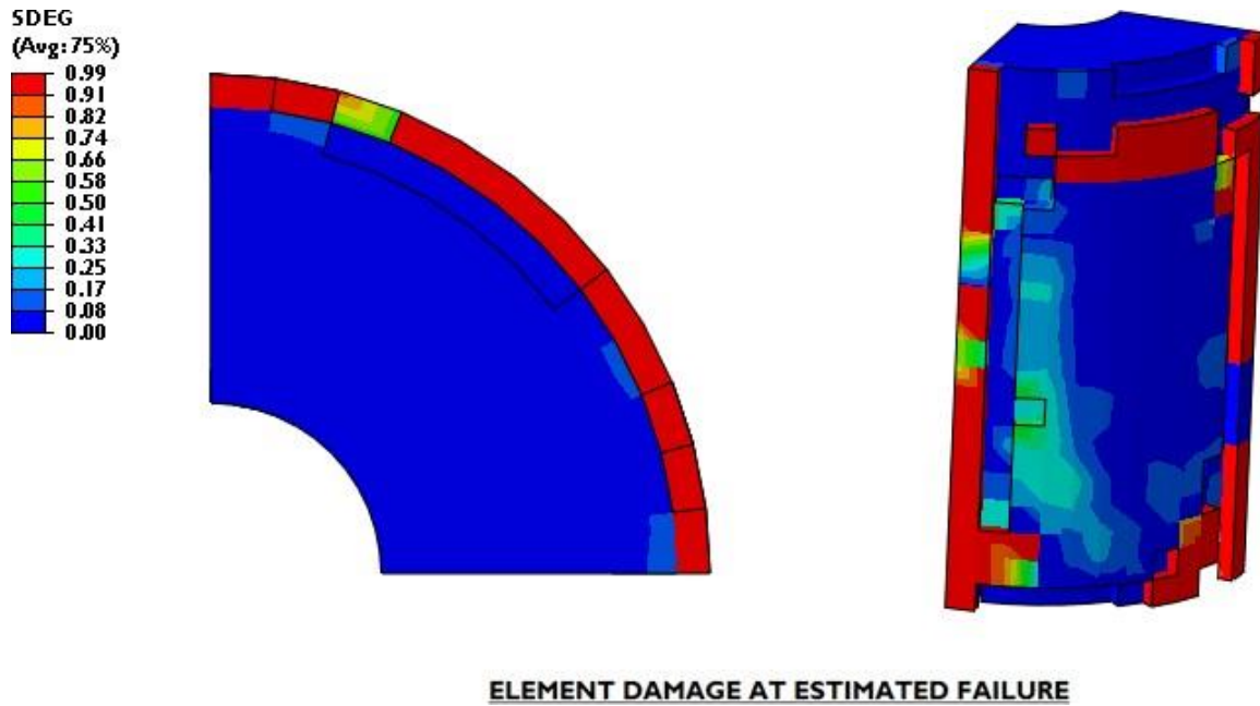
FIGURE 43: CONTACT DAMAGE OF SURFACES IN SMALL SCALE PRESSURE TESTS (CPVC)
